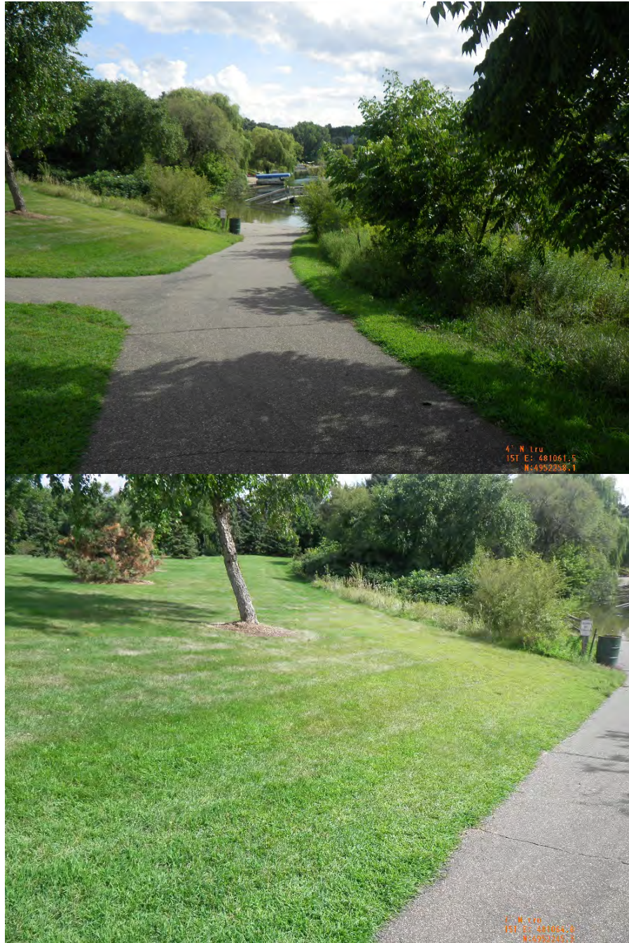
Potential Restoration Area #3 – Stormwater flows directly to the lake along impervious surfaces and turf grass where it can collect pollutants and decrease water quality. Create buffer strips of naturalized vegetation adjacent to the bituminous lake access pathway to slow down and pretreat stormwater prior to entering the lake.
